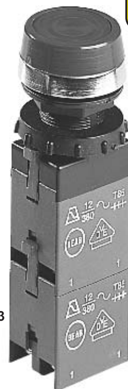
1. 2 x N/O contacts c/w flush pushbutton/chromed bezel for 22.5mm panel hole Product Code: PFY/Colour-P03
